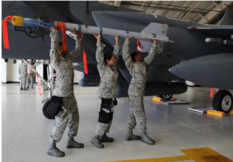
"Crew from the 333rd Aircraft Maintenance Unit attempt to load an AIM-9 Sidewinder missile onto an F-15E Strike Eagle at Seymour Johnson Air Force Base, N.C., Aug. 2, 2012." Image courtesy of
