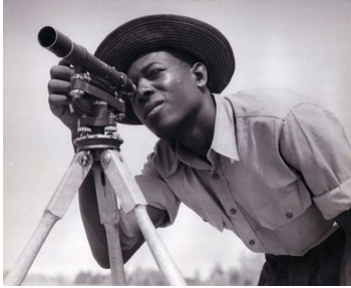
Enrollee sighting through an engineer's level at camp SCS-NC-5, Yanceyville, North Carolina
